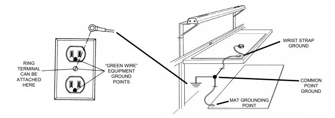
"The single most important concept in the field of static control is grounding. Attaching all electrically conductive and dissipative items in the workplace to ground allows built-up electrostatic charges to equalize with ground potential. A grounded conductor cannot hold a static charge." [Grounding ANSI/ESD S6.1Foreword]
