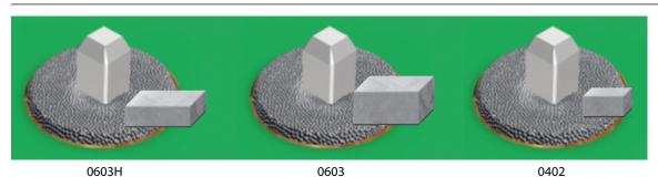
Different chip cap. size solder preforms applied before reflow
