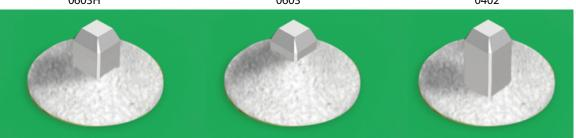
Desired result after reflow, the 0603 chip cap. size creating the largest fillet
