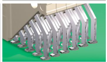
Preforms provide additional solder for tight pitch components and thick PCBs ensuring 100% hole fill and fillet formation.
