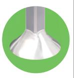
A preform added to solder paste yields 100% hole fill plus fillet.
